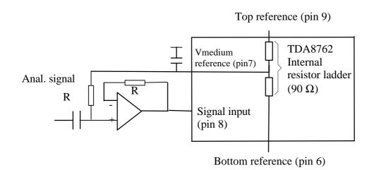
The R resistor in the op-amp loop compensates the offset due to the R resistor connected to Vmed. (R=1k $\Omega$ ; C=1 $\mu$ F)
