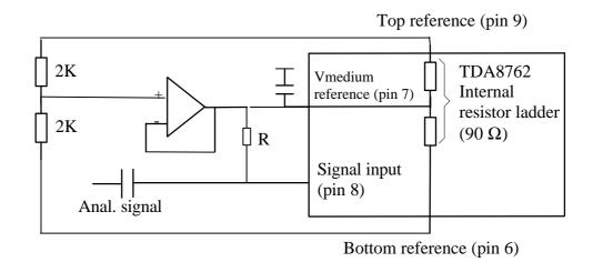
Medium reference is derived from top and bottom reference (input impedance is R // Zin).
