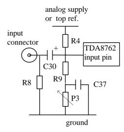
R9 is equal to the output load of the external signal generator. C37 allows ground connection between R9 and P3 in dynamic mode. Typical values when a 50  $\Omega$  signal generator is used are: R4=1K $\Omega$ , R9=50 $\Omega$ ,
