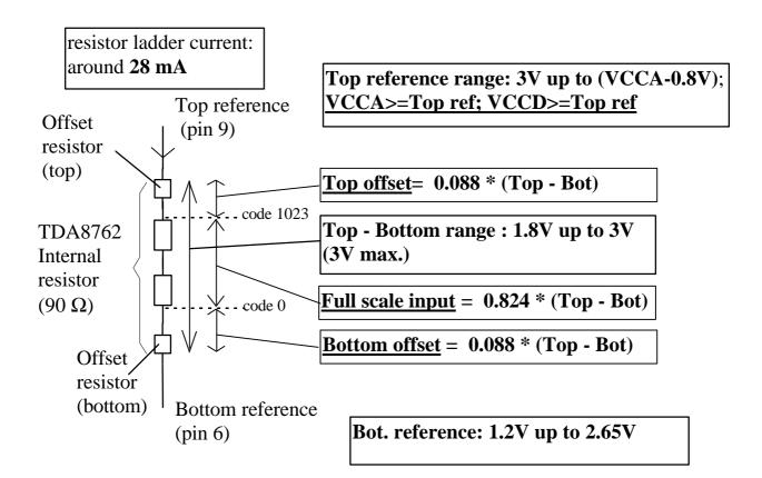
Regulation of the Vtop & Vbottom voltage references depends on the level of cost and quality which are required by the customer application.
