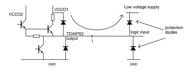
This can happened if a LV logic family is used. The following measurements are obtained with a CMOS low voltage logic family (Philips 74LV04) and they show the current flowing through the protection diode of one input pin:
