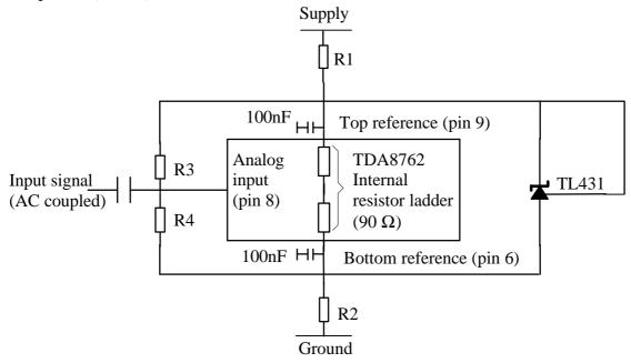
The (top - bottom) difference is set at 2.5V by the TL431, so the full scale input is set at 0.824\*2.5=2.06V. In addition the input offset is set at (Vtop+Vbottom)/2 by two equal resistors (R3 and R4).
