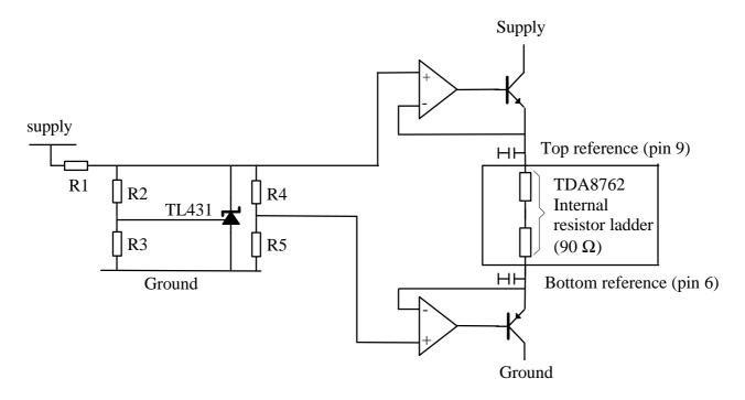
The transistor type depends on the number of TDA8762 mounted in parallel. A 28 mA current (typ) is required for each TDA8762.
