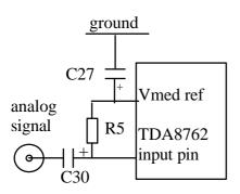
This method gives good results in the following domains: high common mode supply rejection (because both the voltage references and the input offset are derived from the same supply), very low noise level and low cost. R5\*C27 product must be high enough in order to
