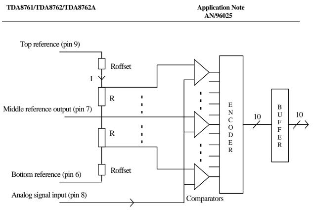
During the A to D conversion the analog input signal (pin 8) is compared to voltage references by using of voltage comparators (in fact these comparators are folding amplifiers).
