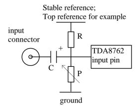
When a resistor bridge is used to provide an offset the current flowing through the resistors must be at least 10 times greater than the signal current (TDA8762 analog input current is 0 to 70 $\mu$ A) in order to guarantee the stability of the input offset. Consequently the resistive value of this resistor string must be below 5.5K $\Omega$  (with a 3.8V top reference).
